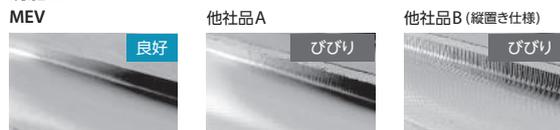
切削条件: Vc = 220 m/min, ap = 3 mm (溝加工), fz = 0.10 mm/t, ø20 (3枚刃), Dry
