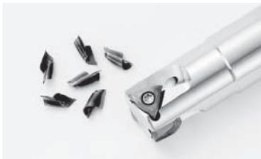
切削条件：Vc = 150 m/min, ap = 6mm (溝加工), fz = 0.2 mm/t, ø20 (3枚刃), Dry
