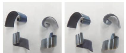
切削条件 : Vc = 150 m/min, ap × ae = 10 × 100 mm, fz = 0.3, 0.4 mm/t, φ125 (1枚刃), Dry 被削材 : S50C
