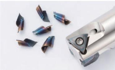
切削条件: Vc = 150 m/min, ap = 6mm (溝加工) fz = 0.2 mm/t, ø20 (3枚刃), Dry 被削材: SS400
