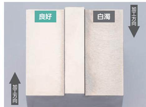
切削条件:  $V_c = 180 \text{ m/min}$ ,  $a_p \times a_e = 3 \times 40 \text{ mm}$ ,  $f_z = 0.1 \text{ mm/t}$ ,  $\phi 50$  (5枚刃), Dry 被削材: S50C
