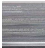
切削条件:  $V_c = 150 \text{ m/min}$ ,  $a_p \times a_e = 3 \times 5 \text{ mm}^2$  4パス,  $f_z = 0.1 \text{ mm/t}$ , Dry S50C ø20 (3枚刃) BT50
